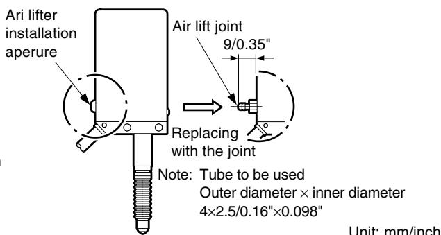
Fig. 2. Using the air lifter (DL310B)
