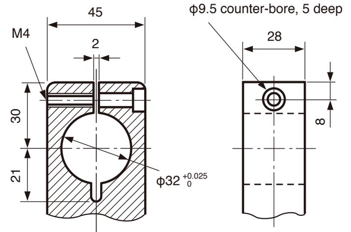
Tightening torque: 6 N·m
