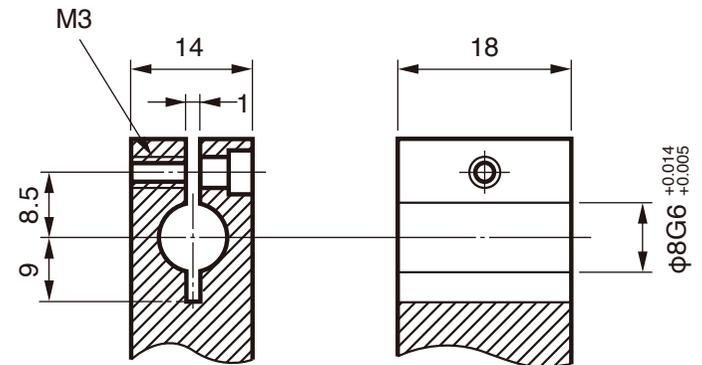
Tightening torque: 0.6 N·m
