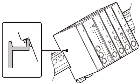
2. Push and install the unit until a click is heard so that the lower side of groove on the back of the unit is fit into the DIN rail.
